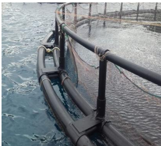
Figure I.4 : Cage flottante (Zaghdoudi, 2013)
